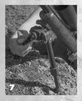
If you encounter a shot at a steep uphill angle. Loosen the tension handle, rotate bipod so logo on the body is facing the shooter. Lower the butt of the rifle while letting the bipod rotate on the spherical ball. Once in the correct position, tighten tensioner. (See picture 7)
