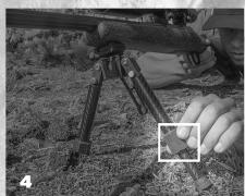
To adjust each leg, loosen the compression collar and adjust legs the desired height, then retighten. (See picture 4)
